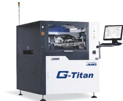
The automated solder paste dispensing reduces production costs by reducing production personnel, dispensing the paste directly from the jar. It extends the solder paste viscosity and maximizes the solder paste lifespan. Additionally, exposure to air is reduced, minimizing issues from improper storage. This also reduces human errors and the chance of mixing old and new solder pastes together.
